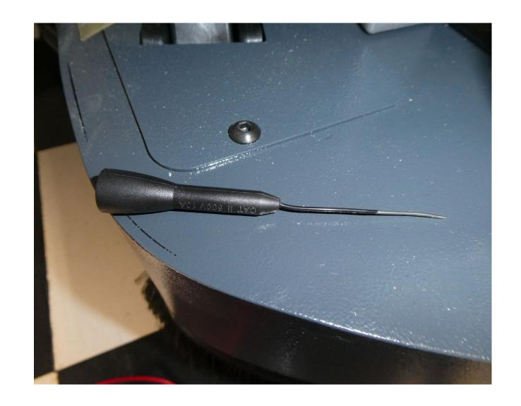
Place your black probe in the terminal block above the Kinetek controller.
