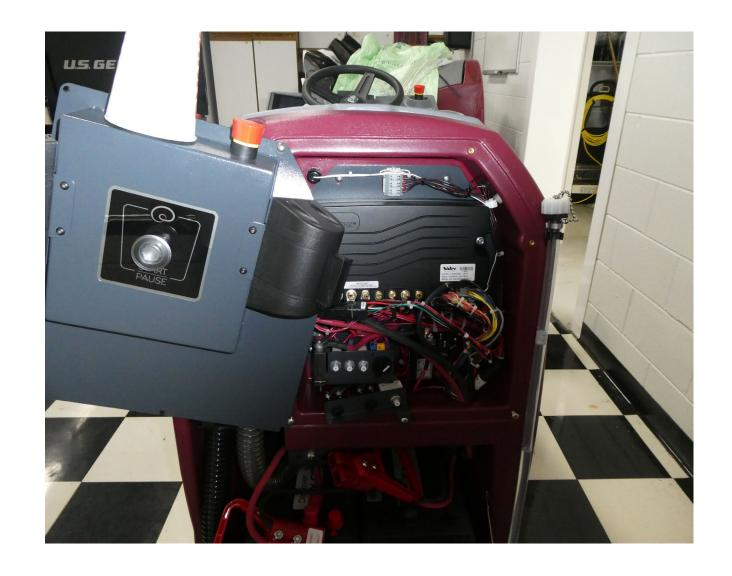
Locate and remove safety tab from Auto/Manual Selector switch.
