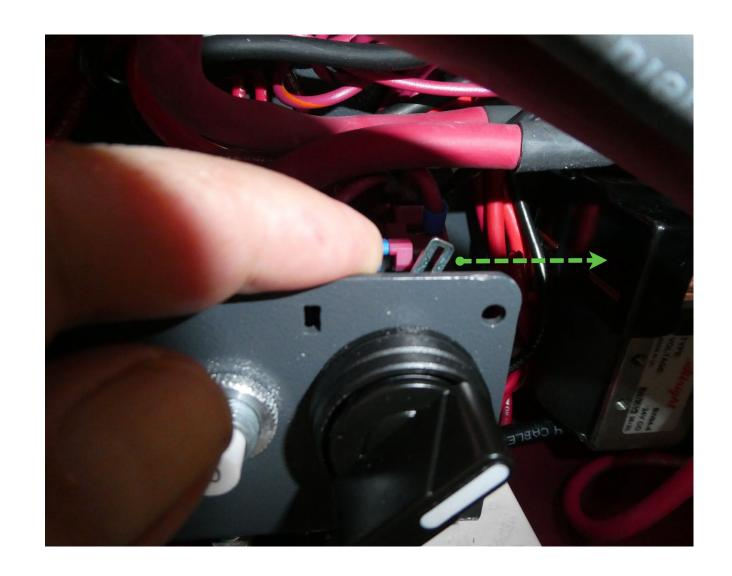
Remove the contact block and bring forward for ease of access.
